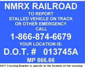
DOT Crossing Number is specific to the location of the crossing The Mile Post (MP) is specific to the locations of the crossing The highway grade crossing posting requires an emergency phone number, the operating railroad's name, the line's MP address and the DOT inventory identification number. There are approximately 211,000 such grade crossings in the United States, each with a unique DOT number.
